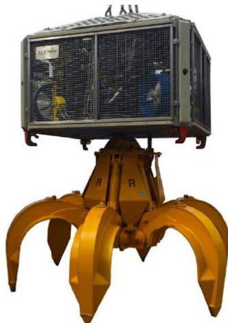
Fig 2 – ROV with integrated grab tool.
