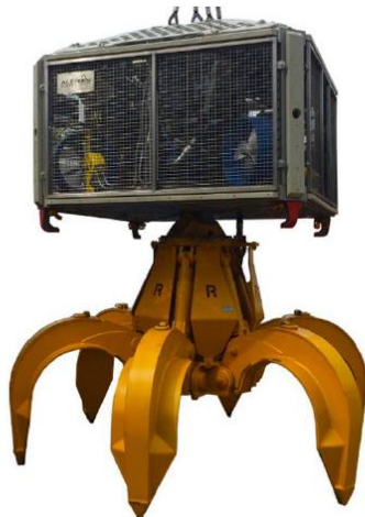
Fig 2 – ROV with integrated grab tool.
